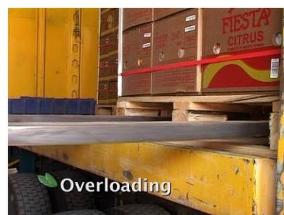
The second scenario is where one of the axles is overloaded because of uneven weight distribution. Incorrect weight distribution of cargo is dangerous because it affects the handling of the truck and may cause accidents.
