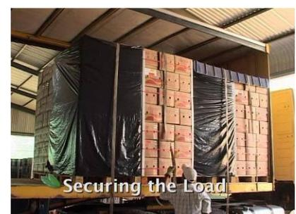
On flatbed and tautliner trucks, there will often be gaps between the pallets at the front of the truck and the front railings of the truck, and on an tautliner also between the back row of pallets and the back of the truck.
